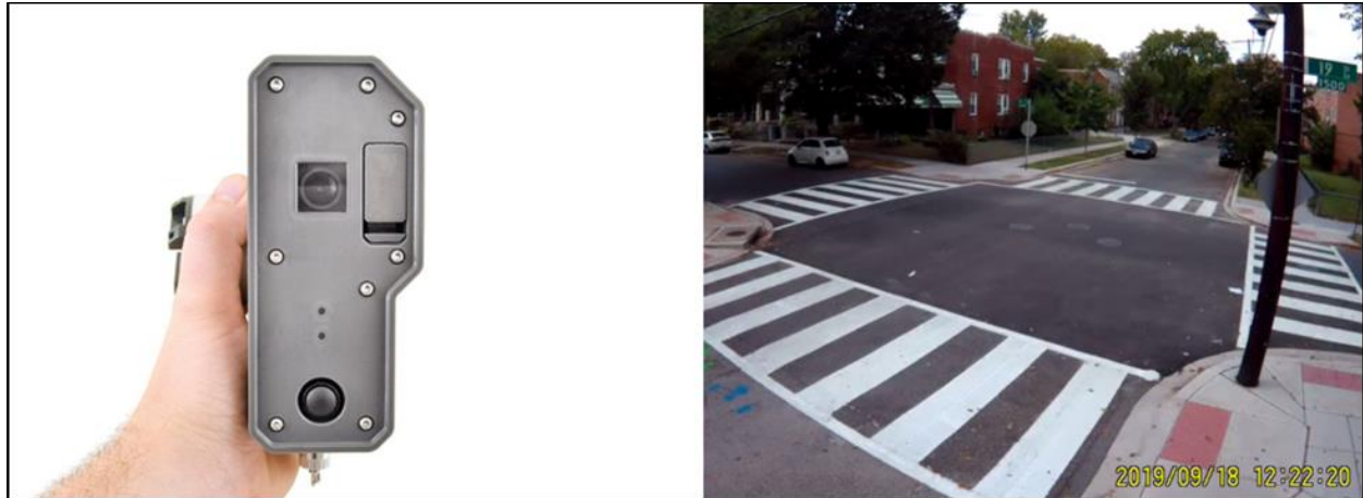
Figure 2: CountCam Video Equipment and Typical Video Playback
